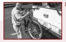
Pull the handle to release and lower the rack. Lower the rack with one hand while holding the bike with the other hand.
